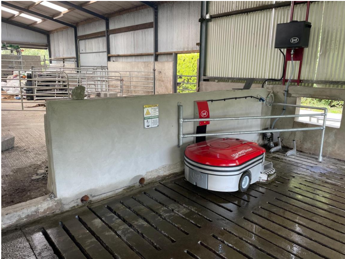
Fig. 10 Permanent structural area needed to facilitate charging, water refilling and deposition of manure
